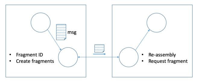
The fragmentation support can operate over a transport using its own fragment/reassembly method (such as TCP), but does not require it, or makes any such assumptions.
